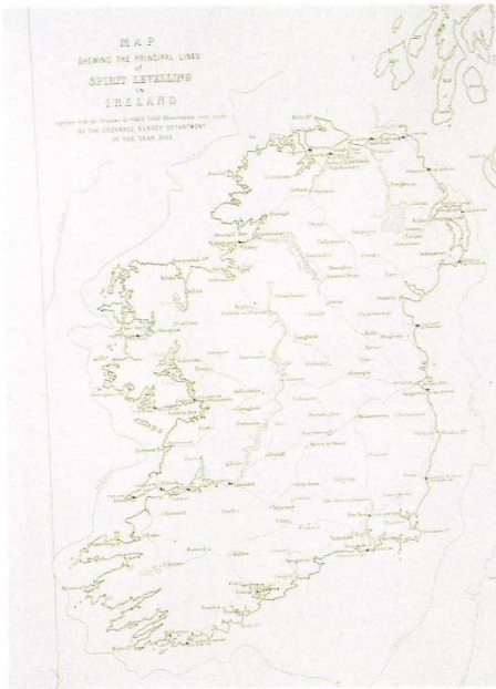
The principal lines of spirit levelling completed in 1843
