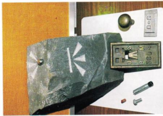
Types of bench marks used by the Ordnance Survey in Ireland
