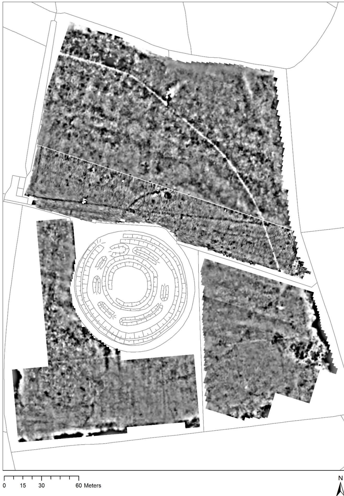
Figure 21 Compilation of the 2006 (Trick) and 2008 (McHugh) electrical resistance surveys which occurred in the same survey area as the 2014 magnetic gradiometry survey.
