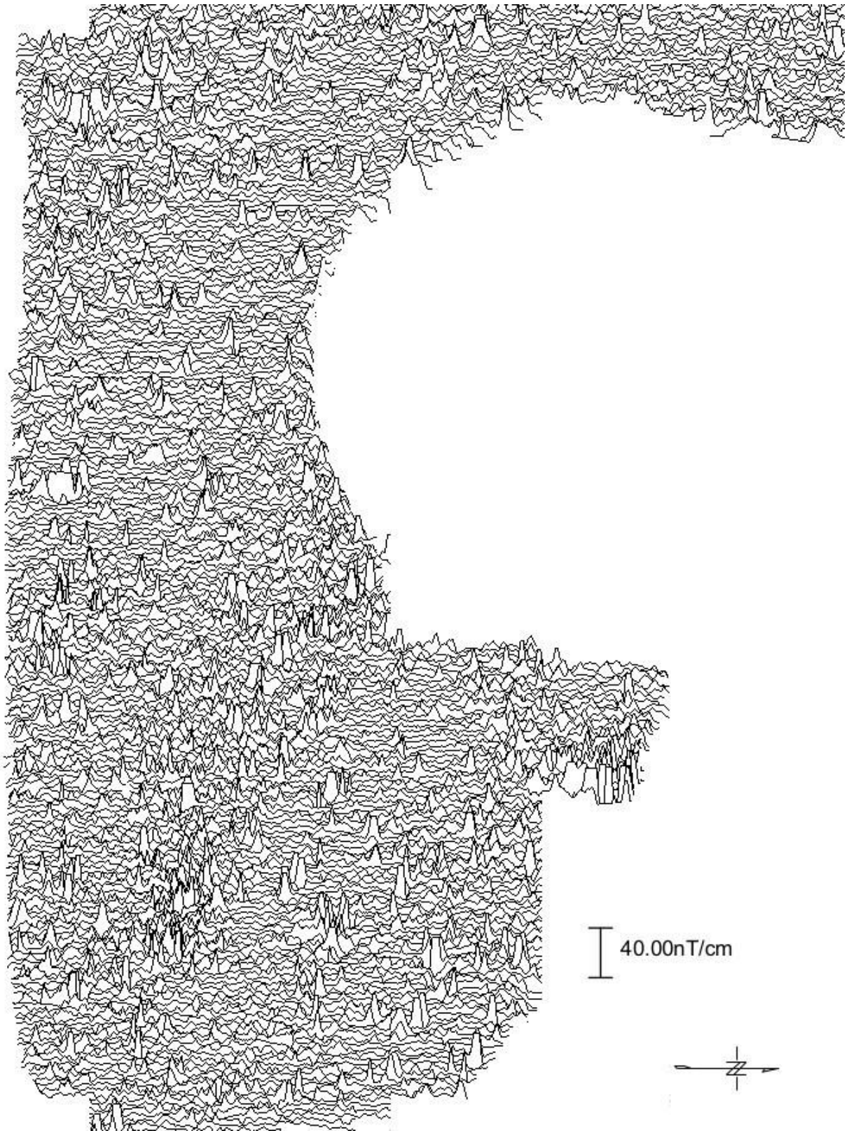
Figure 17 Trace diagram of Area A. Data clipped ( \pm 15 nT) and ZMT (no thresholds).
