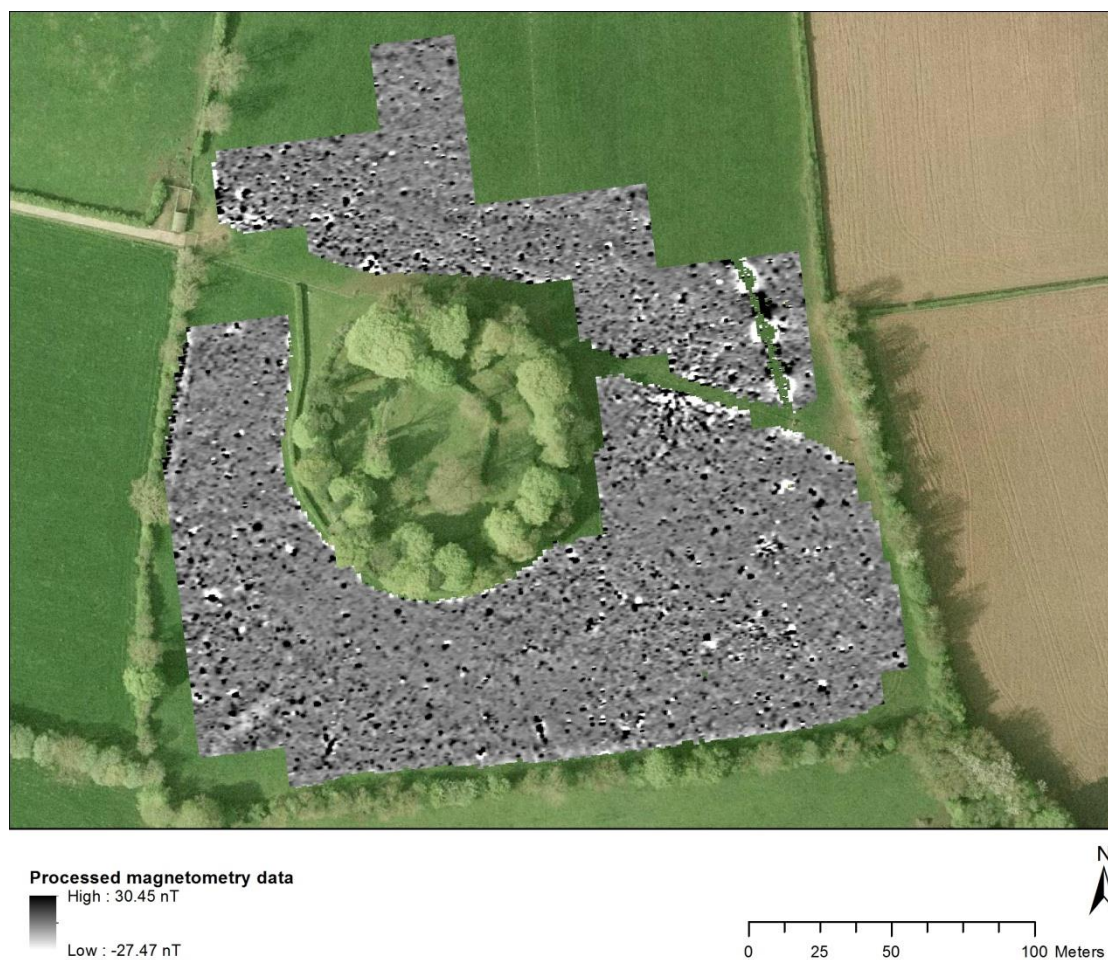
Figure 9: Magnetic gradiometry survey of the scheduled areas to the south and north of the Fort (image provided by Siobhan McDermott CAF).
