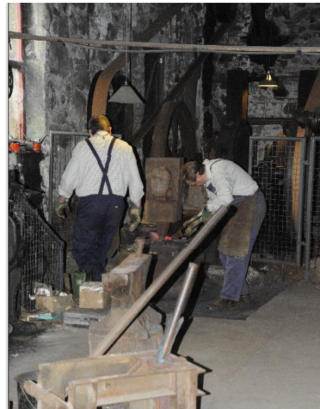
Fig 14. Tilt Hammer in operation at Patterson's Spade Mill (DSC6653)
